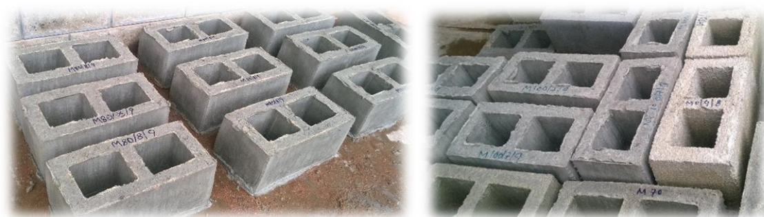
Plate 3:-Blended Sandcrete Blocks: (a) 80% marine sand (b) Various marine-lateritic sand blended blocks.
